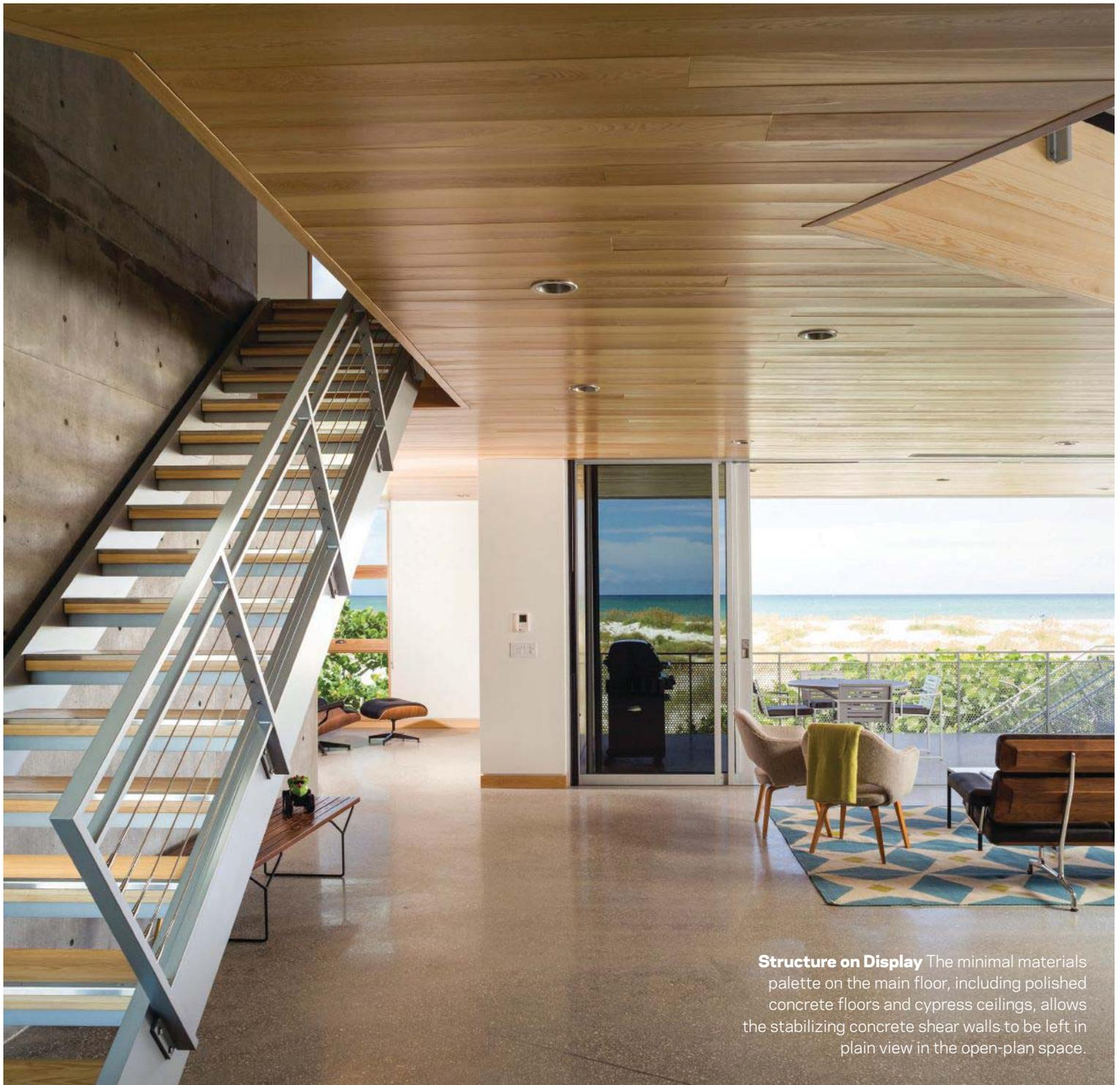
**Structure on Display** The minimal materials palette on the main floor, including polished concrete floors and cypress ceilings, allows the stabilizing concrete shear walls to be left in plain view in the open-plan space.
